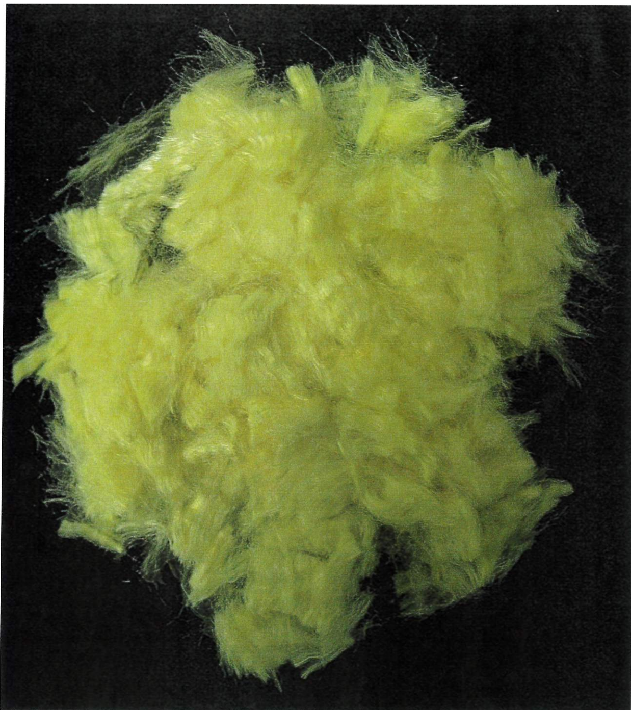
Golden yellow aramid fiber (Kevlar). The diameter of the filaments is about 10 \mu\text{m} . Melting point: none (does not melt). Decomposition temperature: 500-550 ^{\circ}\text{C} . Decomposition temperature in air: 427-482 ^{\circ}\text{C} (800-900 ^{\circ}\text{F} ).
