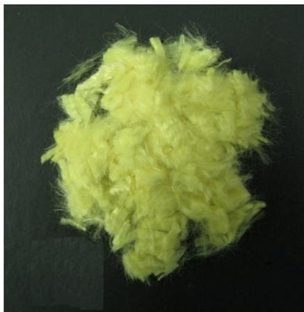
Golden yellow **aramid** fiber (Kevlar®). The diameter of the filaments is about 10 μm. Melting point: none (does not melt). Decomposition temperature: 500-550 °C. Decomposition temperature in air: 427-482 °C (800-900 °F). Author: [Cjp24](#)
