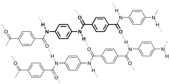
The chemical structure of **Aramid**., Bold: Monomer unit, Dashed: hydrogen bonds. Made by [cacycle](#) (taken from [english](#) wiki).
